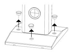
**2.** Place the Kiosk onto the Stabilization Base so that the holes line up as shown.
