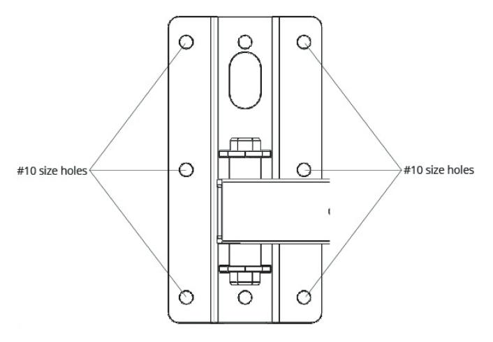
Mounting hardware is included in your package. The screw size for the mounting holes is a #10 screw size. Please research your office's wall type before attempting to install.
